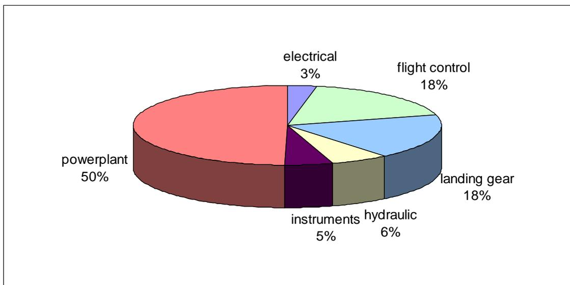
Figure 1: Distribution of system failures among total sample.
